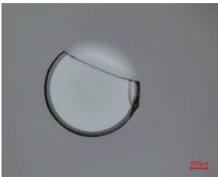
Optical fiber (failed part)
